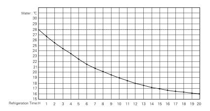
The refrigeration performance test is carried out at an ambient temperature of 30°C without any other additional heat sources.
